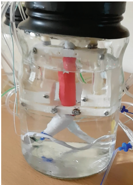
Figure 1. A diagram of the model. 1: a rubber tube 10 cm in length and 1 cm in diameter wrapped with conductive thread to enable the measurement of stress at the walls of the tube. 2: a hydraulic actuator used to apply various longitudinal strain on the tube to simulate ocular distortion during surgical maneuvers. 3: an infrared distance sensor to measure the strain applied on the tube. 4: a sealed container enclosing the model and pressurized to various levels to simulate variable intraocular pressures (IOP). The tests were performed with the container filled with air or water to simulate expansile and non-expansile tamponades, respectively. 5: a pump to pressurize the tube to various levels to simulate systemic intravascular blood pressure (IVP). 6: a pump to pressurize the container to various levels to simulate IOP. 7: a pump to pressurize the hydraulic actuator to various levels to simulate ocular distortion. 8: a pressure sensor to continuously monitor IVP. 9: a pressure sensor to continuously monitor IOP. 10: a microcontroller to control the pumps, process the signals from the sensors and send the information through a serial connection to a computer. 11: a laptop to save and process data from the microcontroller
